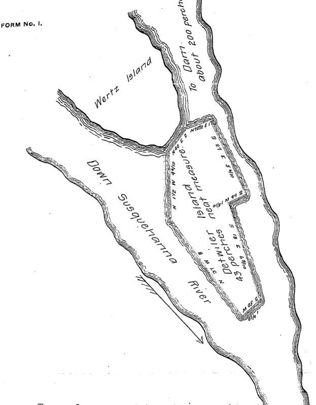
Draft of a tract of Land being an Island containing Forty three perches Strict measure, situate about 200 perches below Columbia Dam, South east of Wertz Island, nearly west of the Red House and North of Rush Island, near the center of the Susquehamna River in Maner township, in the County of Lancaster, Surveyed the 7th day of May 1872, in pursuance of a Warrant granted to Tobias Newcomer & J. W Miller, dated the 2th day of May 1872
